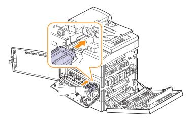
**12** Turn the imaging unit locking levers inwards until it locks in place and close the inner cover.
